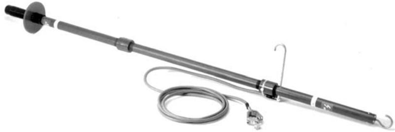
**Figure 8: A typical discharge and grounding stick. The end hook applies a resistance to discharge the UUT, and the side hook applies a direct ground connection.**
