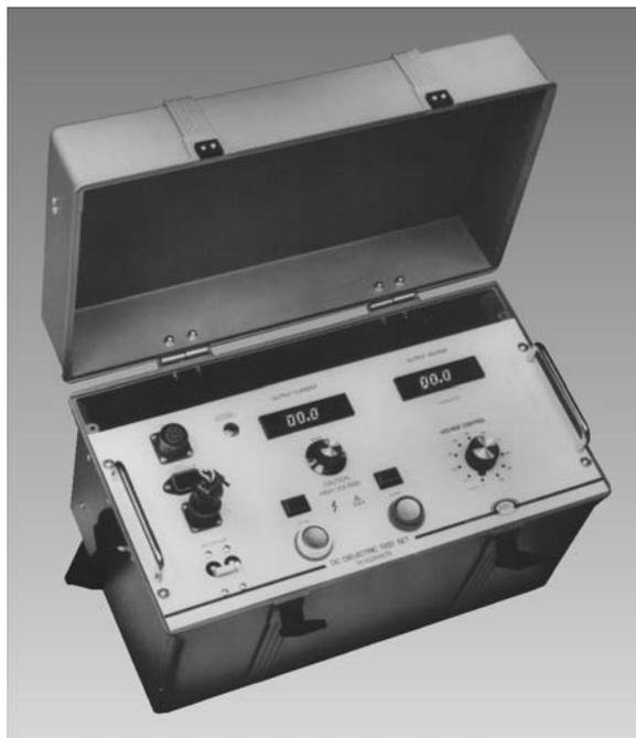
***Figure 5: Control Unit of 70 kV, 120 kV or 160 kV dc test set***
