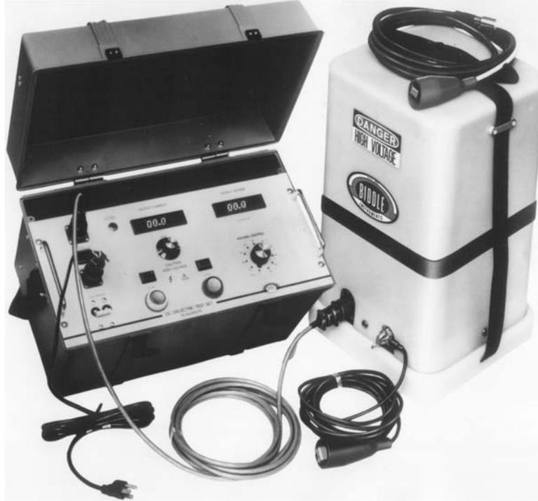
***Figure 7: A 70 kV dc test set, which is available with analog or digital metering. Two other models offer test voltage up to 120 kV or 160 kV.***
